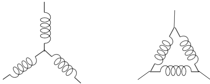
Figure 2-10 Star (left) and delta (right) connections
