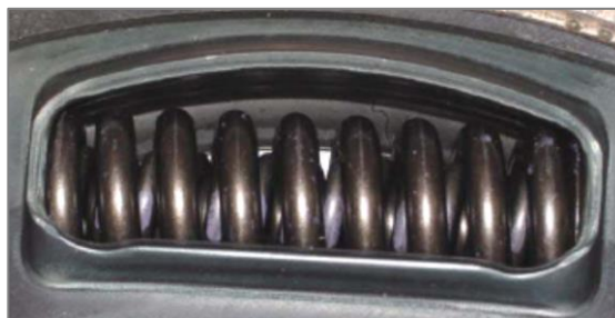
Figure 2.9: Typical LTD helical coil spring in damper eyebrow pocket [28]
