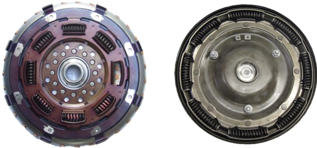
Figure 2.8: Left - Coil spring LTD TCC damper, Right – Linear spring (curved pocket) TCC Damper [30]
