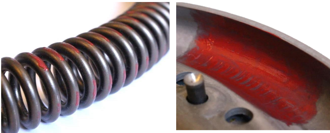
Figure 6.2: Assessing outer spring contact with its housing (secondary inertia)
