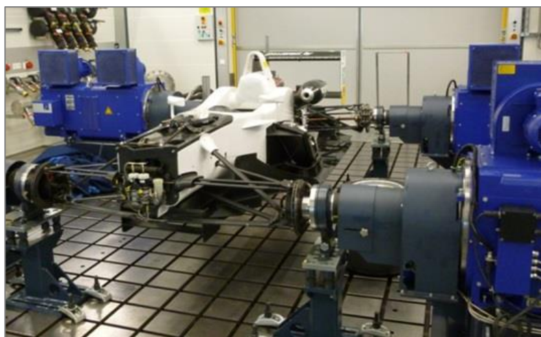
Figure 2.19: Full powertrain and driveline modular test facility [46]
