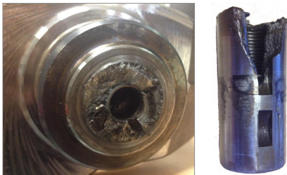
Figure 4.15: Failure of crankshaft snub nose end (pulsation generator input)
