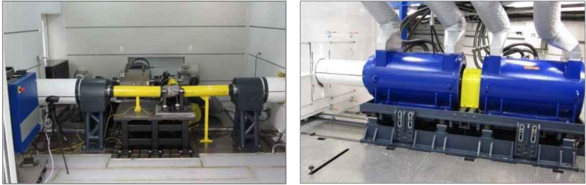
Figure 2.17: McLaren Durability & NVH test rig – inside the acoustic chamber (Left) & the external motors (Right) [38]
