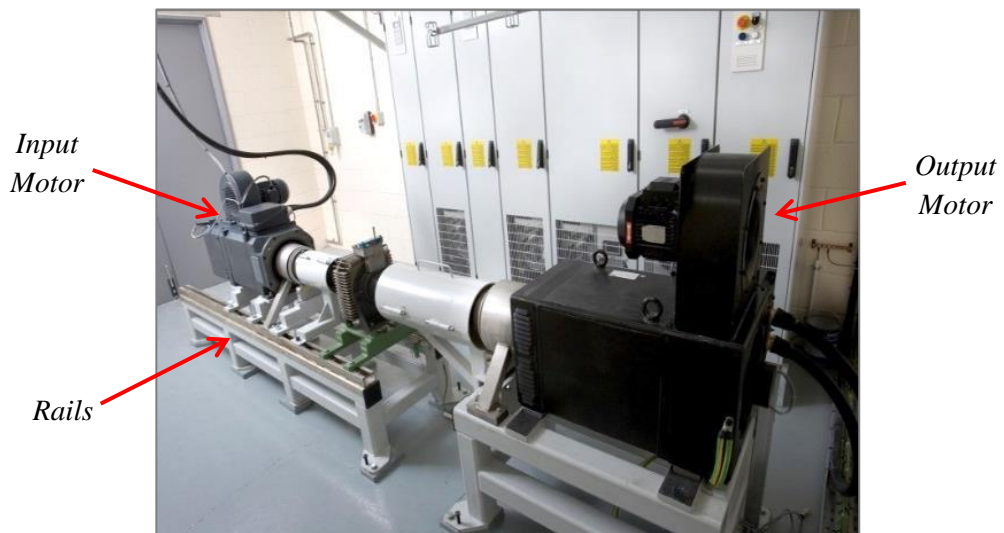
Figure 3.1: PVRC rig before torque converter testing upgrades
