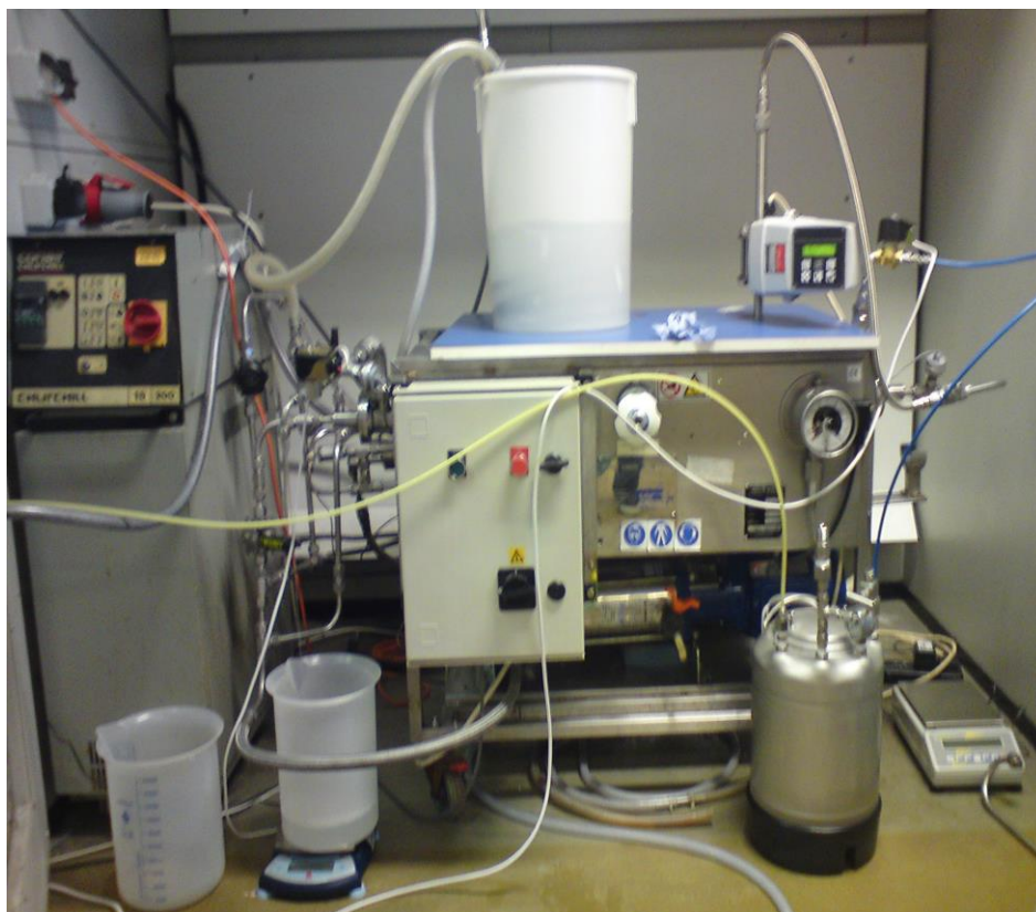
Figure 33. Photograph of the newly constructed filtration system (set-up 3)
