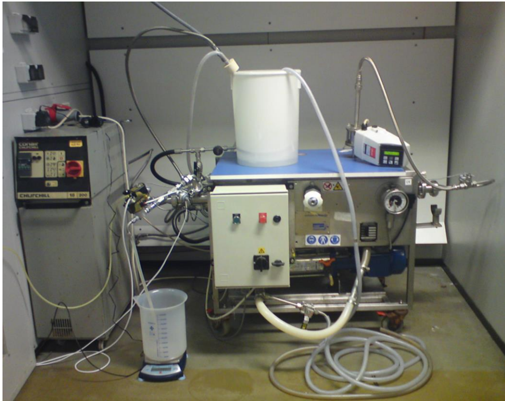
Figure 31. Photograph of the newly constructed filtration system (set-up 2).
