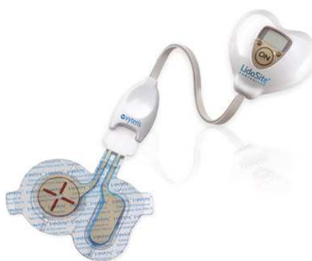
Figure 4. The LidoSite ™ iontophoretic system for topical delivery of lidocaine ( http://www.vyteris.com/home/Our_Products/Lidosite.php )
