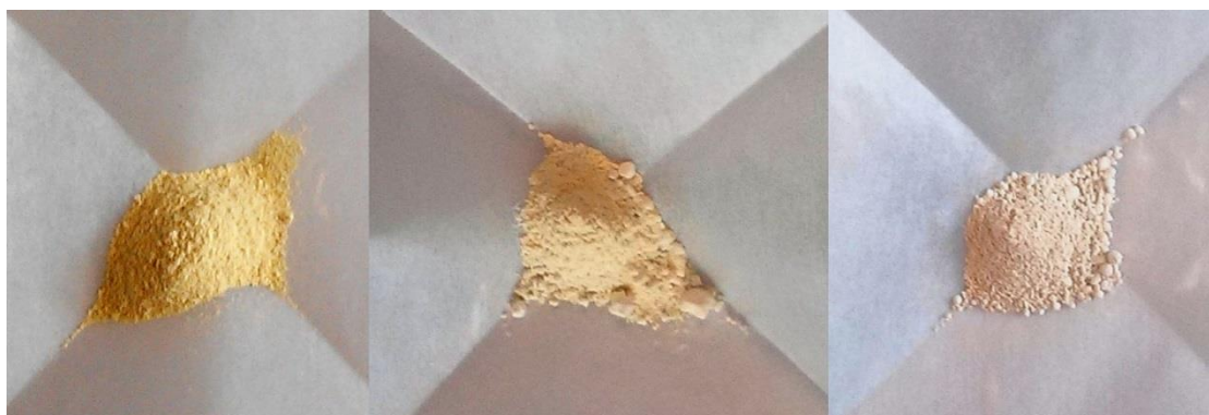
Figure 4.1 – Photographs of ceria nanostructures, showing the progression in colour from yellow to white. From left to right the nanostructures are CeNP, CeNR A and CeNC A .
