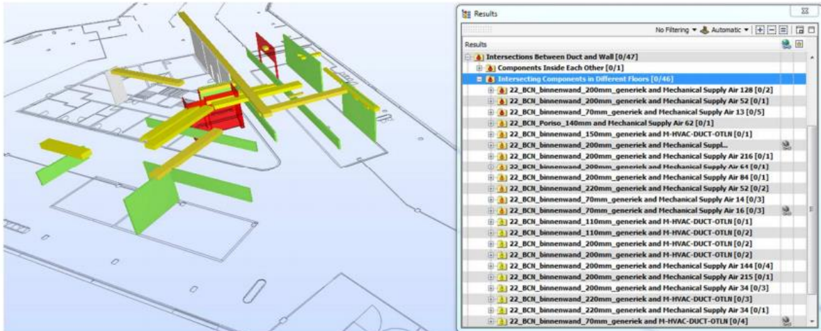
Figure 101 Automatic visualization of identified objects conflicted with asbestos (Zijlstra, 2014)
