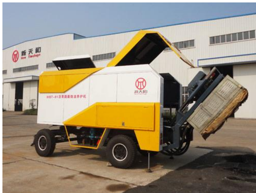
Figure 163 Asphalt repair Microwave heating mechanism
