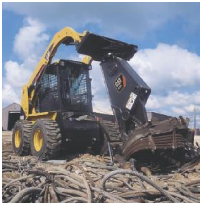
Figure 184 Hydraulic large size shear machine
