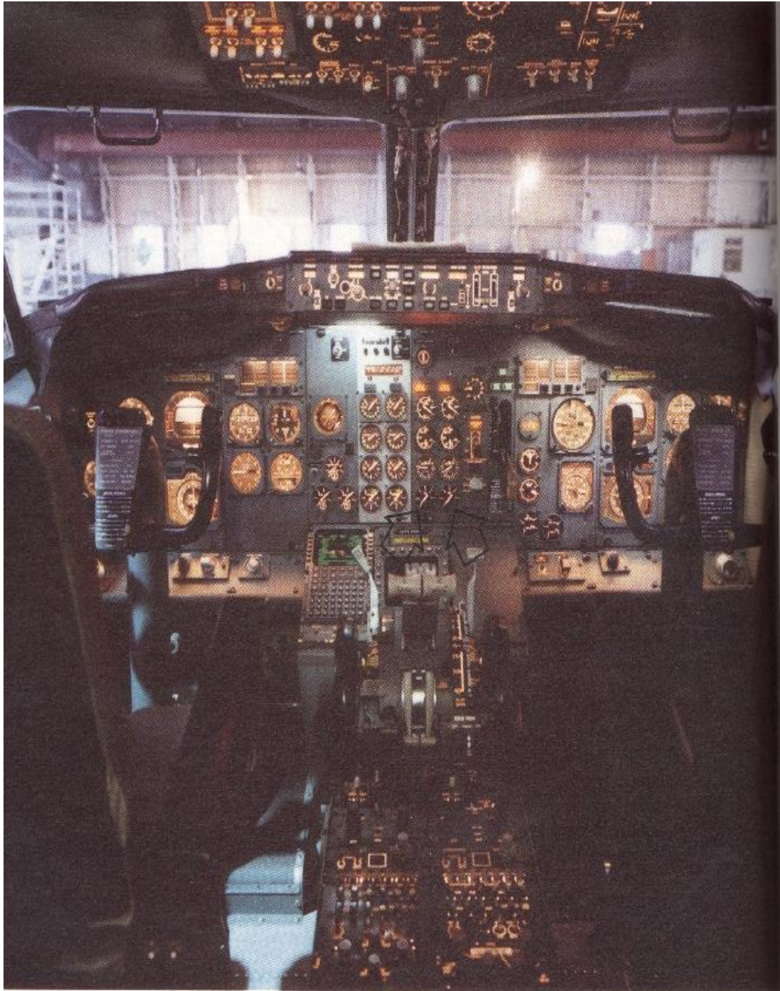
SHOWING HYBRID ELECTROMECHANICAL POINTER/LED COUNTER INSTRUMENTS USED FOR DISPLAY OF ENGINE PARAMETERS WITH VIBRATION INDICATORS ARROWED
