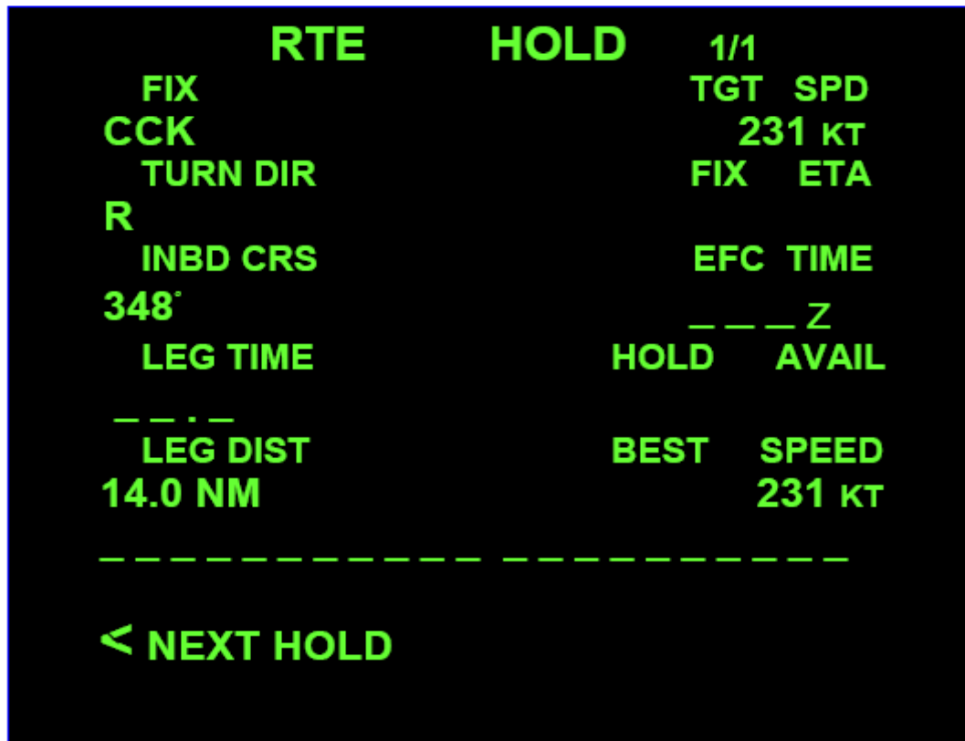
Figure 5.3 FMC CDU display showing hold page after the leg distance had been entered.
