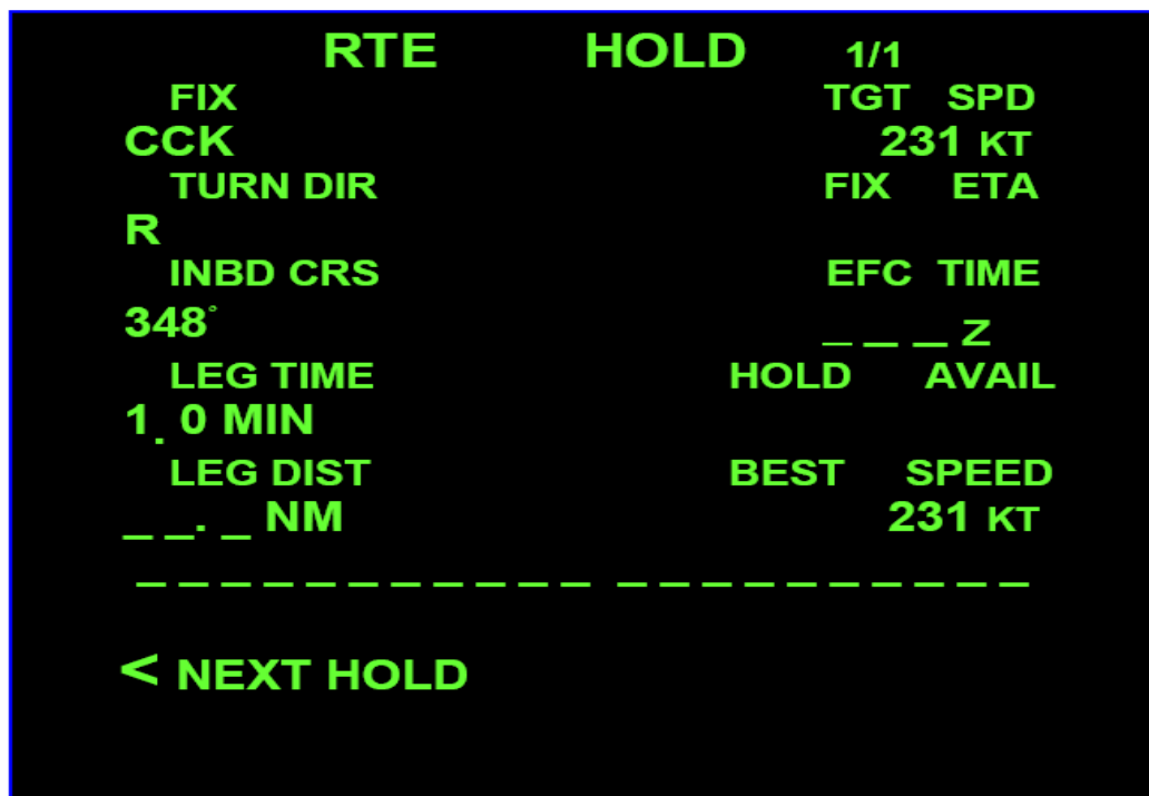
Figure 5.2 FMC CDU display showing hold page before the leg distance had been entered.
