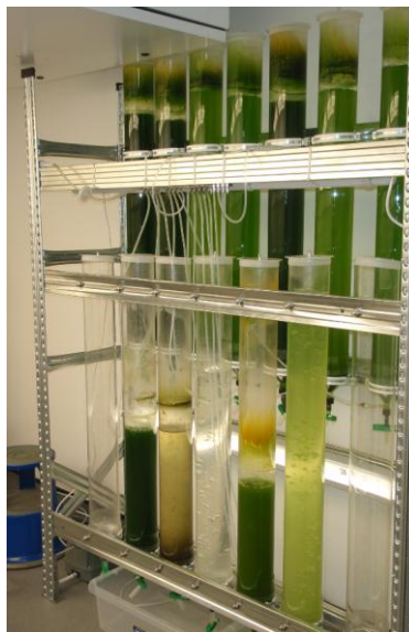
Figure 2.3: The 8l 'ExAlga' vertical photobioreactors (vPBR) in the Fitotron ® plant growth room. These vPBRs were used for the production of larger quantities of biomass of C. emersonii .
