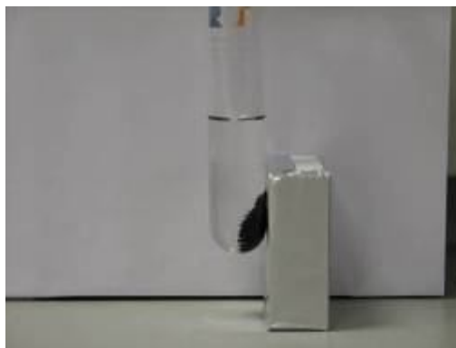
Figure 6. Quick separation using permanent magnet.
