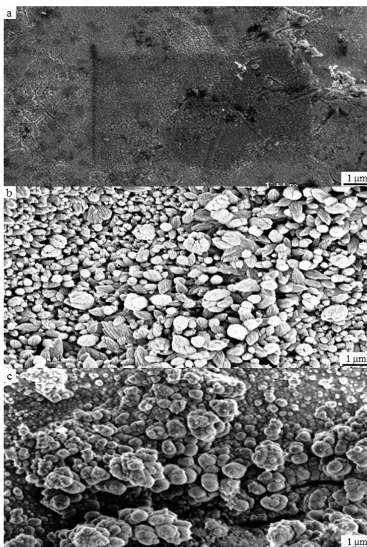
Figure 5.22 FESEM micrographs of Zn foil exposed to different external environments. Zn foil exposed to air (a); Zn foil immersed in deionised water (b); Zn foil immersed in deionised water with UV irradiation (c).
