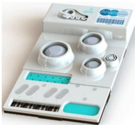
Figure 2.2: Multichannel cartridge developed by Atlas Genetics
