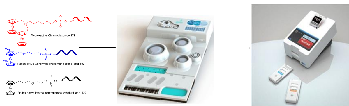
Figure 4.16: Triples DNA detection assay developed being used on the commercial cartridge set up at Atlas
