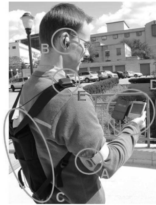
(b) SenSay prototype, showing wearable hardware, from [125].
