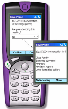
(a) BayesPhone , which performed context inference in real time (using probabilistic context models learned offline), from [98].
