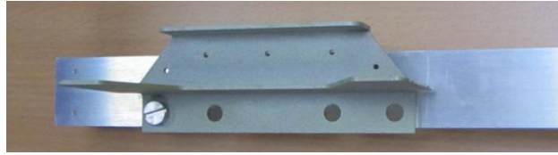
Figure 74: T-cleat and lower wall bracket. Datum pin in position that provides precision location for panel.
