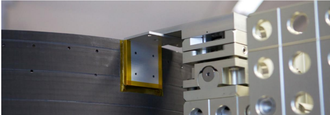
Figure 79: Cylinder brackets bonding tooling used for all brackets to reduce tooling and improve assembly accuracy through reduced setting variation.
