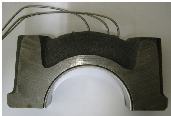
Figure 5.36 – Crank cap instrumentation with shell bearing in position
