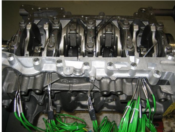
Figure 5.38 – Crank cap thermocouple cables routing out through ladder frame and cylinder block interface
