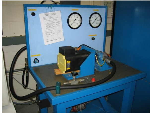
Figure 5.27 – Hydraulic test rig showing variable speed motor and pump
