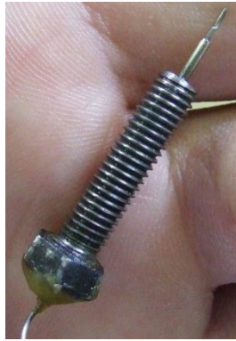
Figure 5.24 – Thermocouple mechanical fitting used by Nottingham University
