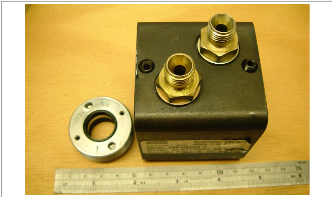
Figure 5.8 Hydraulic cylinder with end removed.
