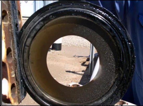
Figure 2.7. Wet black powder in orifice plate [145].
