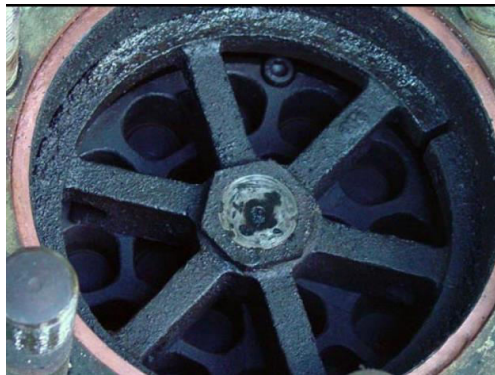
Figure 2.11. Compressor valve with black powder coating [145].
