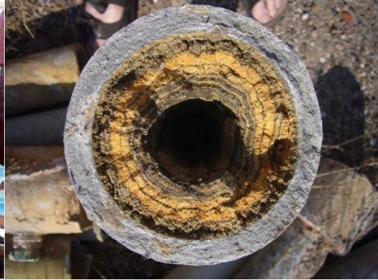
Figure 2.2. Mineral scale in a pipeline [127].
