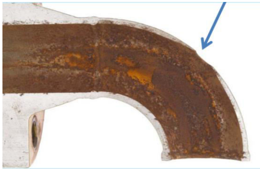
Figure 2.10. Erosion caused by sand particles to (a) a 50 mm bend pipe and (b) a choke valve [144].
