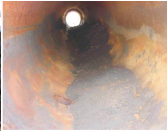
Figure 2.5. Black powder in a 508 mm pipeline [95].
