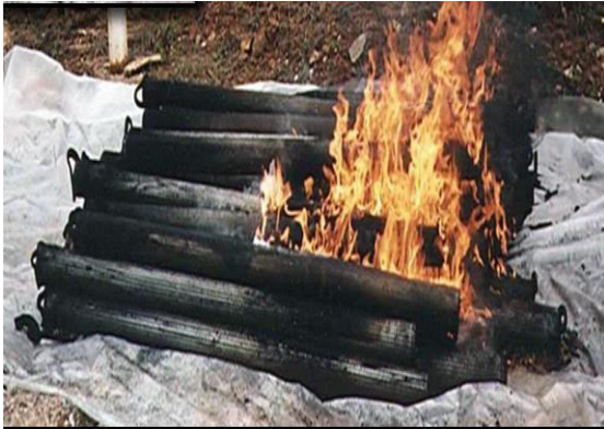
Figure 2.8. Pyrophoric iron sulfide fire [145].
