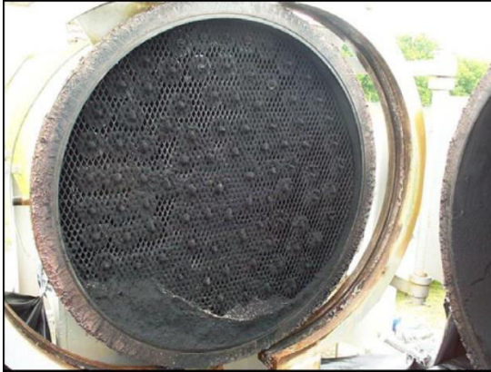
Figure 2.6. Filter coated with black powder [145].
