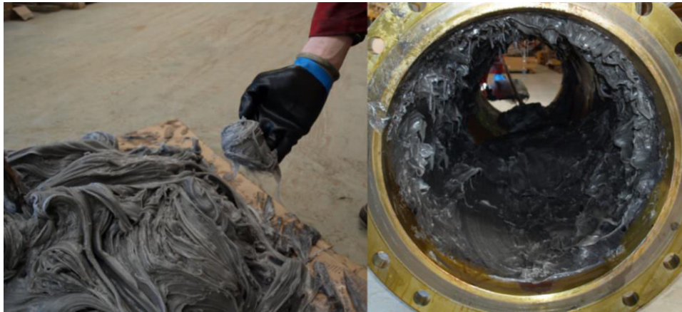
Figure 2.3. Wax formation in an oil pipeline [143].
