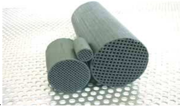
Figure 7. Activated carbon monolith (Crittenden, et al. , 2005b)
