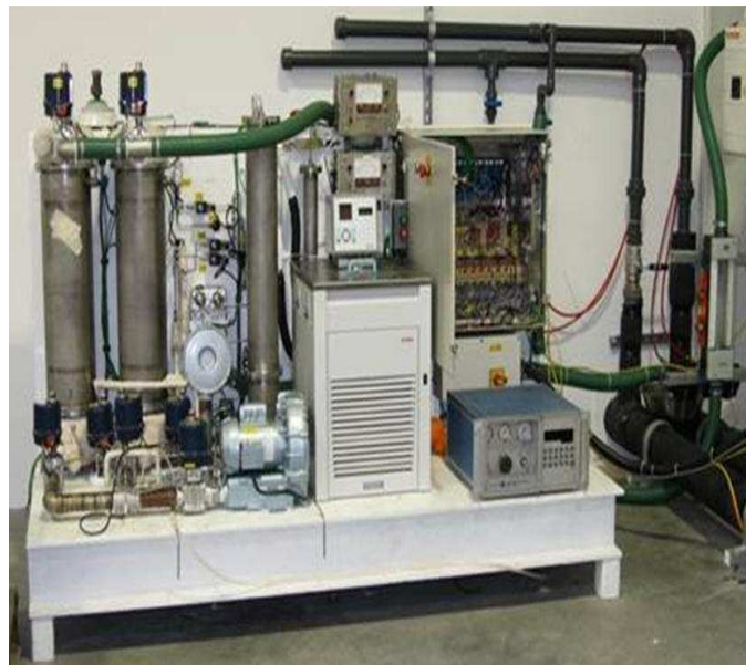
Figure 106. First commercial ACM fast cycle solvent recovery unit (Crittenden, 2011)
