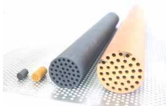
Figure 13. Green and carbonised monoliths (Crittenden, 2011)
