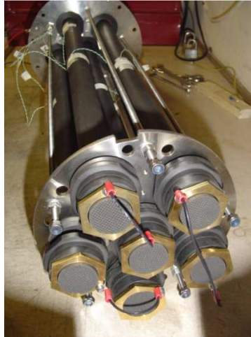
Figure 10. ACMs assembled into a module and electrically connected (Crittenden, 2011)
