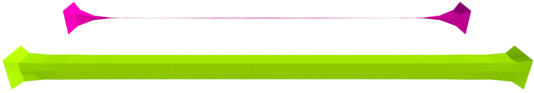
Figure 5.1: Comparison of volume constraints. Meshes using our volume constraint (foreground) and the co-rotational pressure term \text{tr}^2(\mathbf{R}^T \mathbf{F} - \mathbb{I}) (background) are stretched to 2.5x their original length. The standard term causes the mesh to lose 90% of its volume; the mesh using our constraint gains 1.2%. Such strains are not uncommon in simulation of flesh deformation, so the benefits of an accurate volume constraint are clear in that case.
