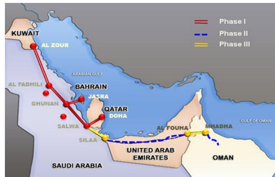
Figure 1-2: GCC power grid commissioning phases[5]
