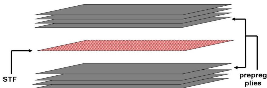
Figure 87 - Schematics of STF/CFRP composite preparation
