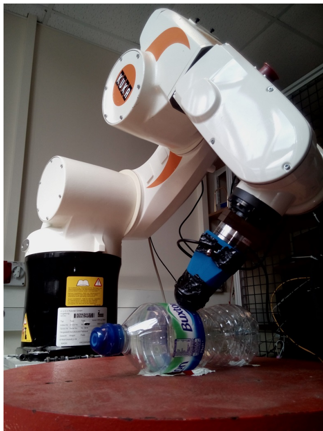
Fig. 1. Tactile data is collected autonomously by the tactile sensor developed in [7], mounted on a KUKA KR-650.
