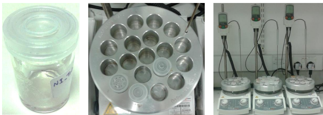
Figure 2.10 Temperature controlled evaporative crystallisation carried out in 7 mL glass vials using custom designed DrySyn ® holders (Asynt Ltd.) on hotplates at a range of temperatures, allowing the parallel exploration of a range of crystallisation variables.
