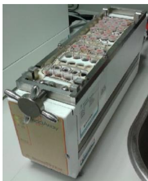
Figure 2.11 ReactArray Solo Microvate reaction block for temperature-controlled crystallisation.
