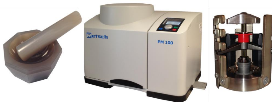
Figure 2.14 Apparatus used for mechano-crystallisation.
