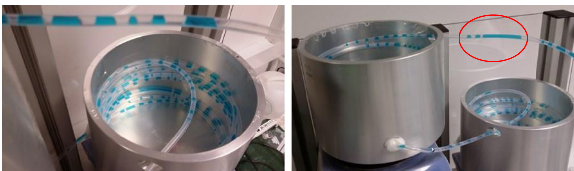
Figure 6.11 Photos of irregular segmentation of methanol (coloured with methylene blue) using PFPE as carrier fluid. The red ring highlights a large slug created by Ostwald ripening.
