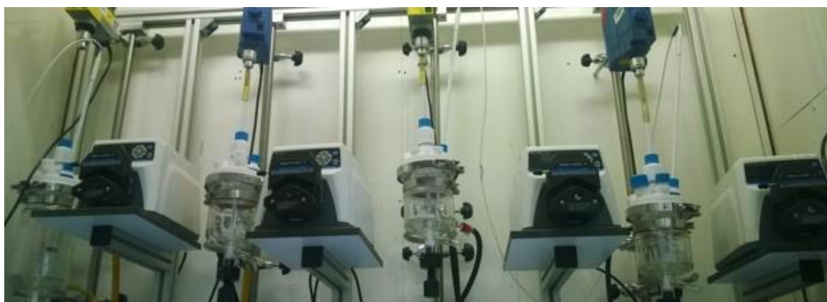
Figure 5.5 Photograph of the MSMPR set-up (from left-feed vessel, nucleator and growth vessels 1 and 2) used in experiments carried out within CMAC at Loughborough University (LU).
