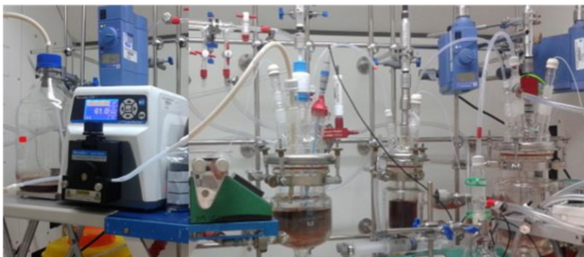
Figure 5.20 Photograph showing the set-up of vessels used in UBA MSMPR experiments at AstraZeneca, Macclesfield.
