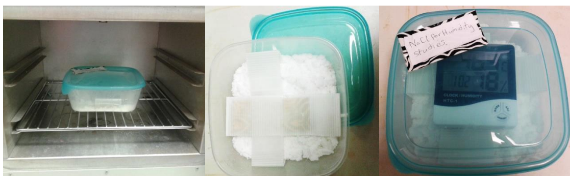
Figure 4.9 Rudimentary set-up for long term humidity exposure testing comprising airtight container, sodium chloride and water mixture, plastic shelf to hold materials and a humidity sensor
