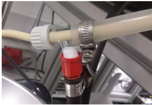
Figure 6.20 Flexible tubing jacket developed to prevent fouling in transfer lines between the feed vessels and mixer piece.
