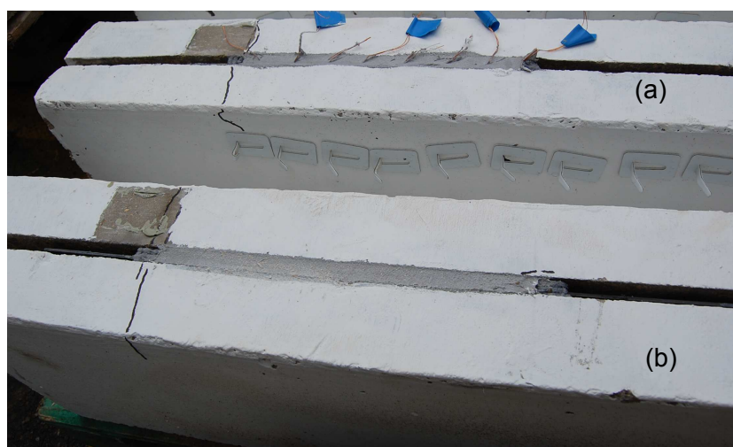
Figure 4.10 - Specimens (a) 8-31[R/60/L/6.4p] and (b) 8-31[R/60/L/6.4p] control with no strain gauges (no damage in the resin or the concrete in both specimens)
