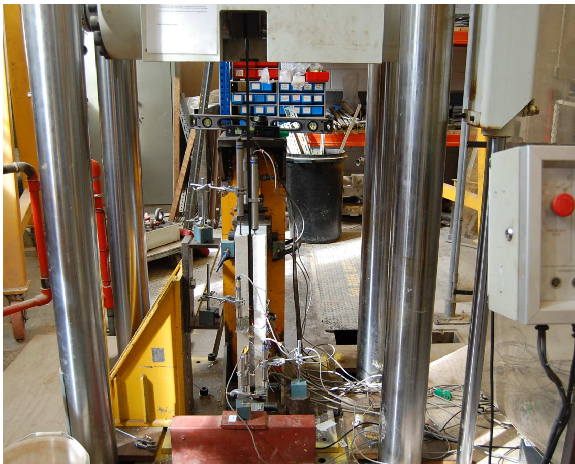
Figure 3.17 - Bond test set-up
