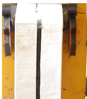
Figure 4.13 - Tensile rupture in specimen 8-31[R/60/L/6.4p]control with no strain gauges
