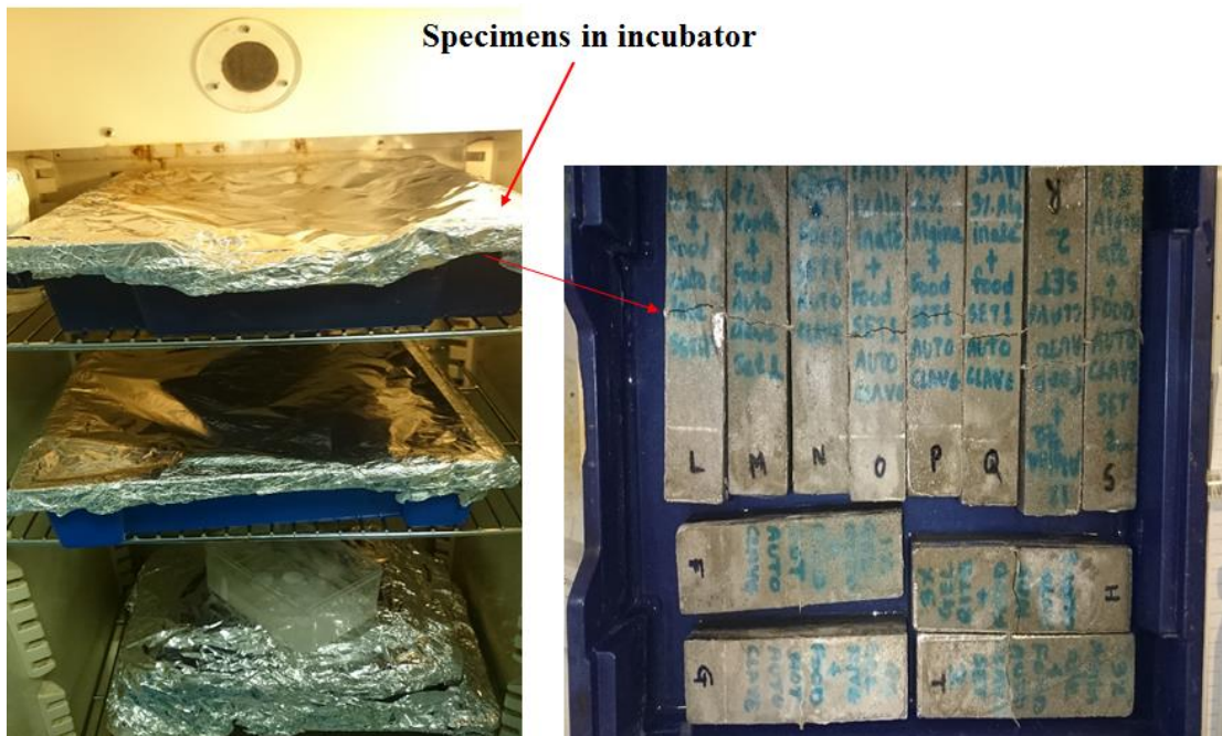
Figure 8.12: Samples with bacterial and bacterial self-healing agents incubated at 30°C.
