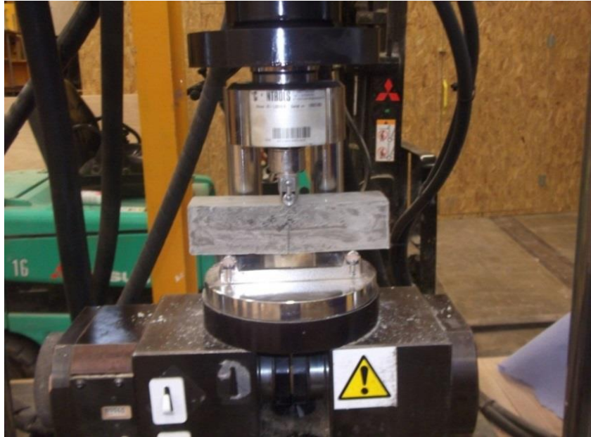
Figure 4.3: 3-point bending test machine.
