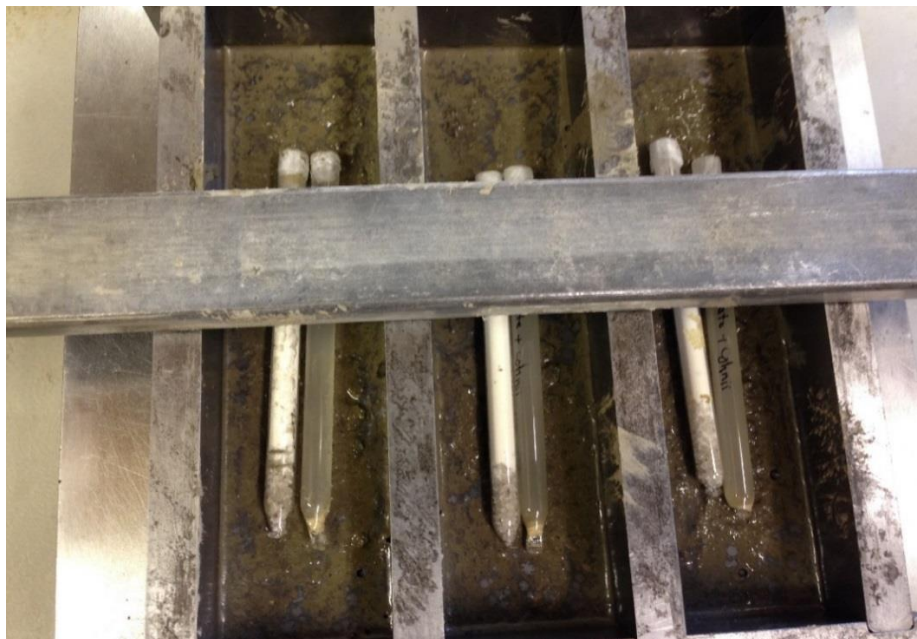
Figure 8.14: Preparation of glass tubes with bacterial and bacterial self-healing agents during casting of samples.
