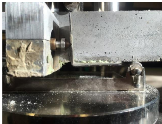
Figure 7.1: 3-point-bending test with LVDT sensor.
