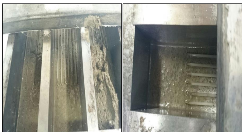
Figure 8.10: Shows capillary glass tubes preparation during casting of samples.
