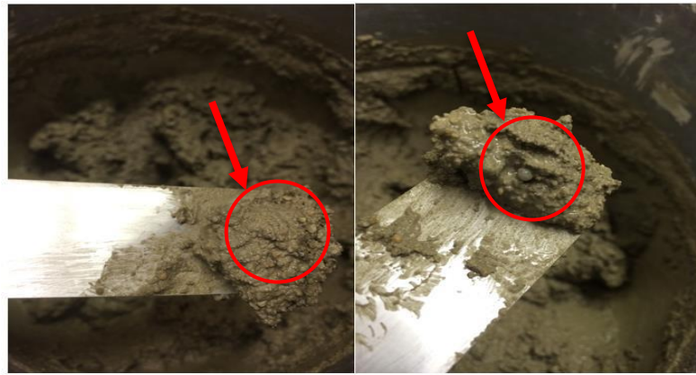
Figure 8.5: Shows calcium alginate beads during mix with mortar paste.
