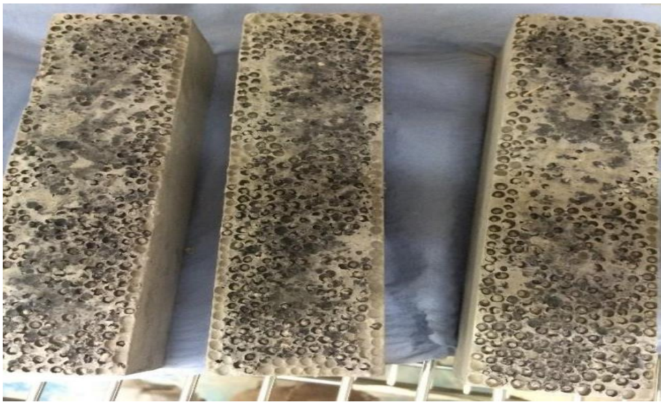
Figure 8.9: Cross-sections of calcium alginate bead mortar samples after 24 hours in the conditioning room.
