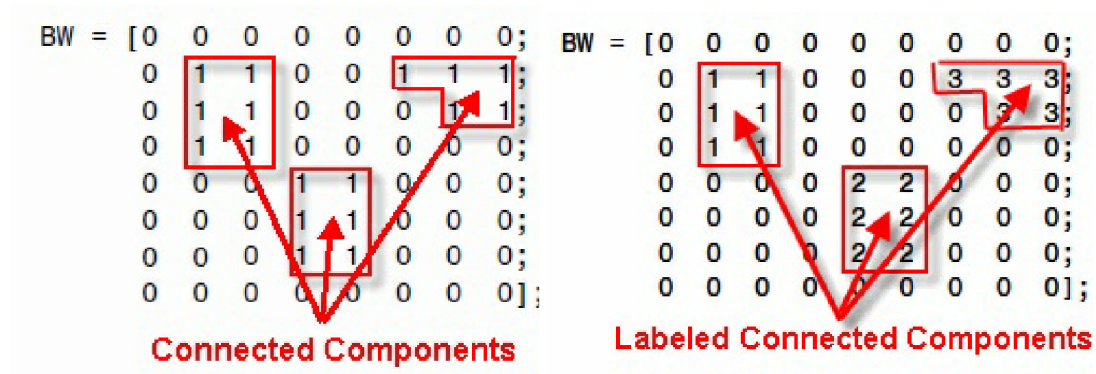
Figure 4-17: Left: An example of connected components in a binary image with three connected components. Right: An example of labelling connected components in a binary image. Connected components in the binary image are identified before being a new unique label
