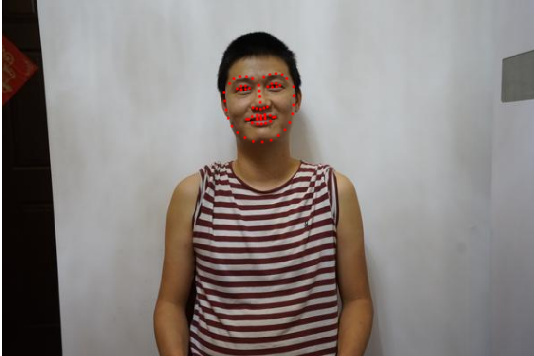
Figure 3-9: An example of facial landmark detection result
