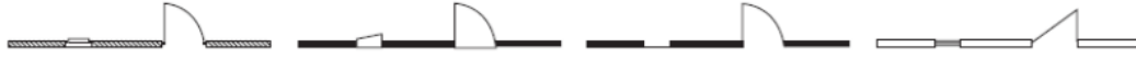
Figure 4-1: Different ways to draw a wall with a window and a door. The variable graphic symbols pose challenges for automatic recognition of objects in CAD drawings. [163]
