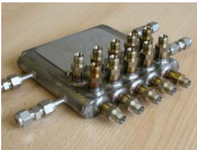
Fig. 1.1 Structured compact reactor-micro heat exchanger used in this work.
