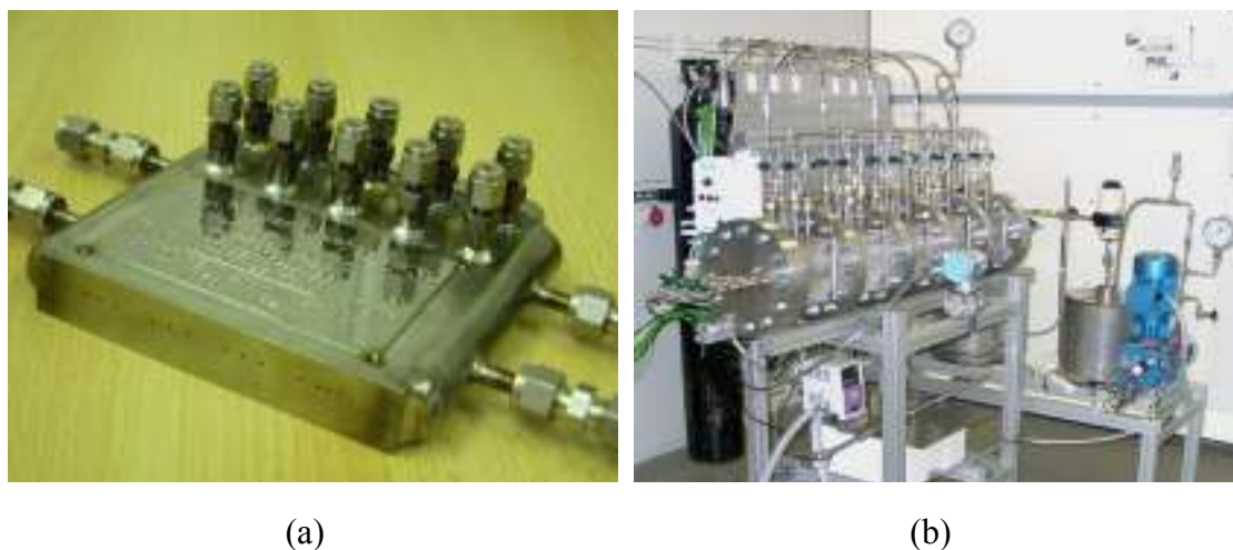
Fig. 2.6 (a) Structured compact reactor with mm-scale reaction channels, (b) the pilot-scale compact reactor (192 of 500 mm length, 3 mm i.d. channels, up to 150 t/a liquid throughput).
