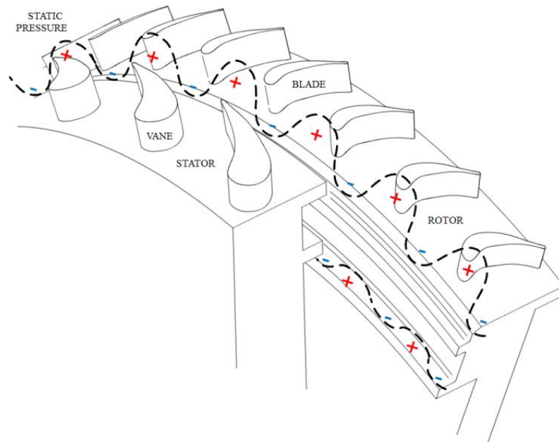
Figure 3.12: Variation of static pressure in a turbine annulus. Red and blue indicate regions of high pressure and low pressure with respect to the wheel-space, respectively. For the double rim-seal shown, the pressure asymmetry is attenuated in the outer wheel-space between the two seal clearances.
