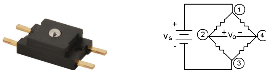
Figure 57: Honeywell FSS1500-NSB force sensor used in the fin test rig.
