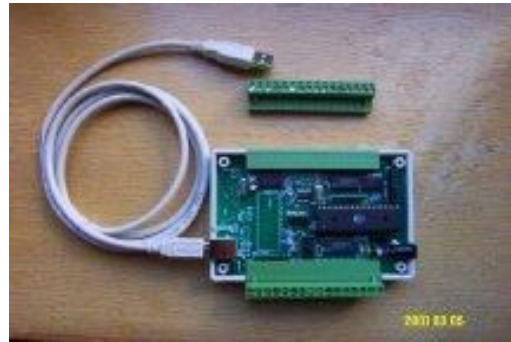
Figure 127: normDAQ-5003 quadrature encoder counter module (USB version).
