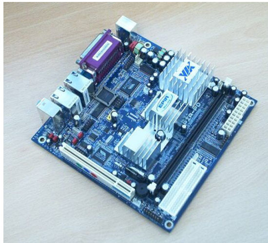
Figure 122: EPIA-PD6000E motherboard used in the Bathymysis submarine.
