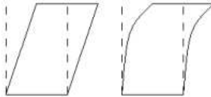
Figure A-3: Possible variance in centre of mass of seal during flexing motion
