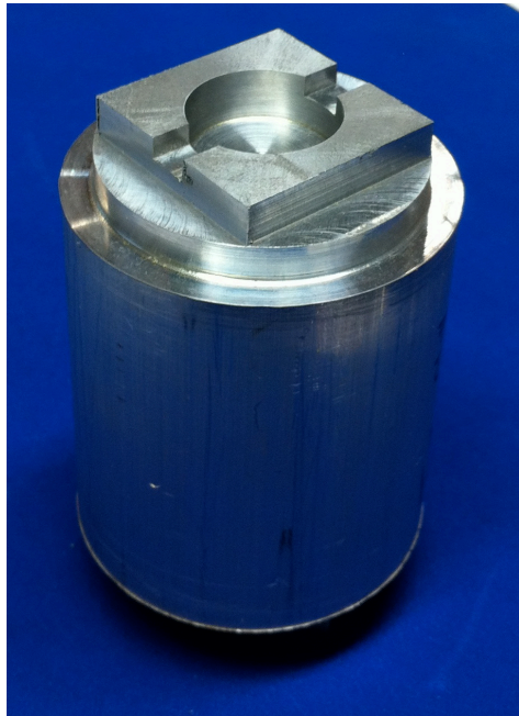
Figure 7.13: Finished turn-mill part
