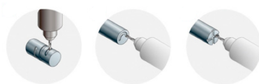
Figure 3.28: Capability of controlling C-axis (Mas.Tech., 2013)
