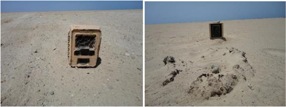
Figure 2: Painted camera with wooden box.
