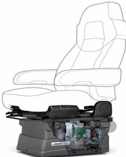
Figure 2-12: Bose active seat system [78]
