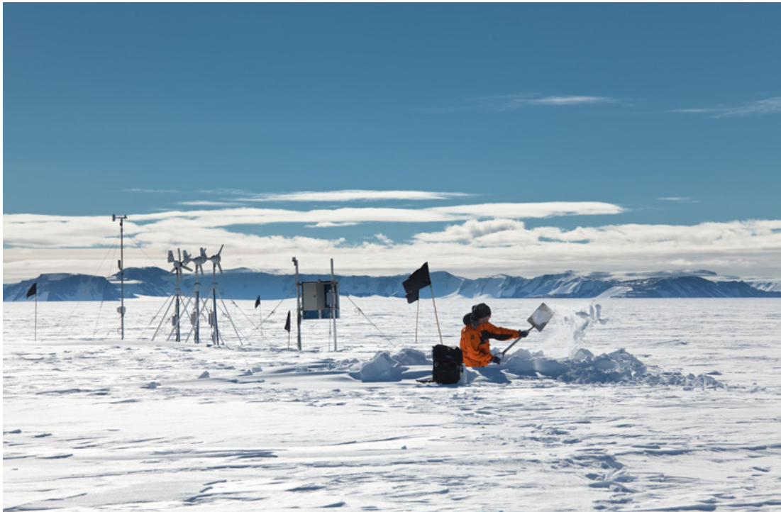
Figure 10.1 – A remote Antarctic GPS scintillation monitoring station at Site Eagle (81°S). The power support system can be seen in the background alongside an array of wind turbine generators and an automated weather station mast. The author can be seen digging out the GPS receiver box, which is buried to protect the electronics from harsh surface wind temperature fluctuations. The GPS antenna is out of shot in the foreground, a sufficient distance away from the wind turbine blades – a potential source of multipath interference. This PhD research has relied heavily on remote measurements and sustained operation from the Antarctic receiver network.
