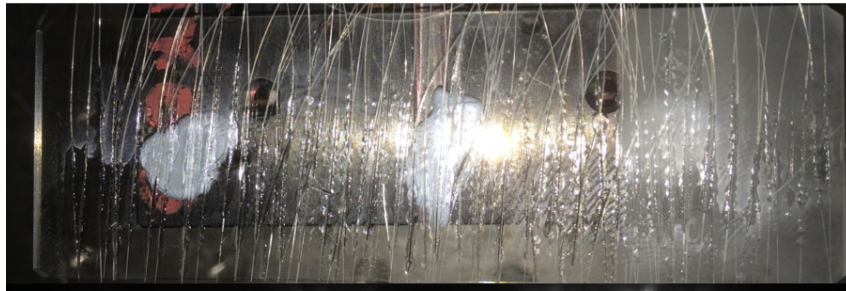
Figure 10-6 Reduced cladding fibres glued on a microscope slide and then cleaved at the end forming a multifibre output in one plane. The fibres are not equally spaced.
