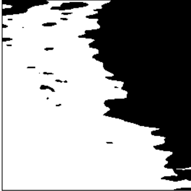
Figure 5.18: Output mask for the Land test case using FSFS with 1 feature and 2D GFB (4,6,0)
