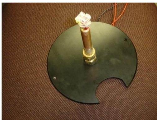
**Figure 4.7** LED's wired through metal tube mounted onto back-plate
