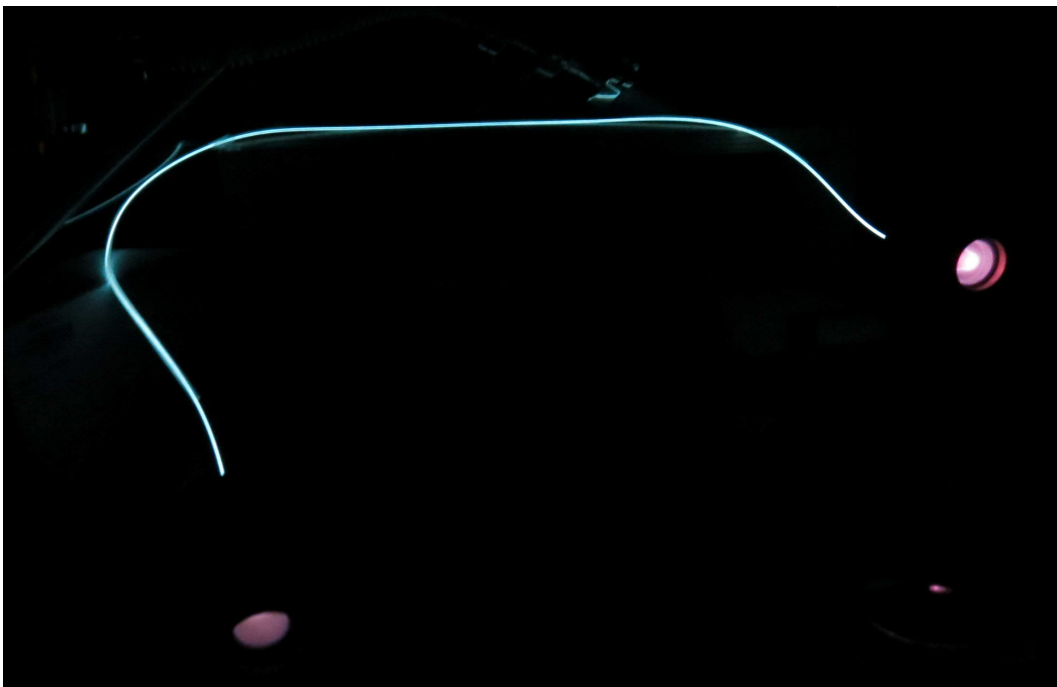
Figure 5.11: Photograph of a helium-xenon discharge 1 m in length. The high voltage anode glow is on the left, with the cathode glow on the right.
