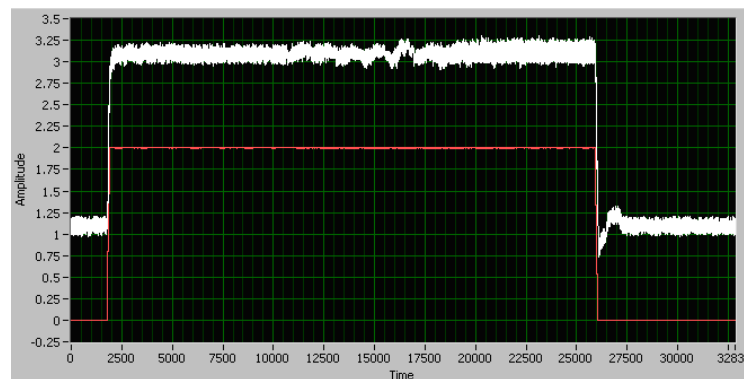
Figure 5-38 – Solenoid profile when leaving a gap of 0.5cm between the toe pad and the load-cell contactor. -
