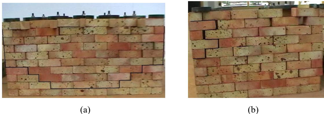
Figure 4.20 The response of Model II on y-axis 1.8Hz 12mm excitation ((a) the façade; (b) the side wall)
