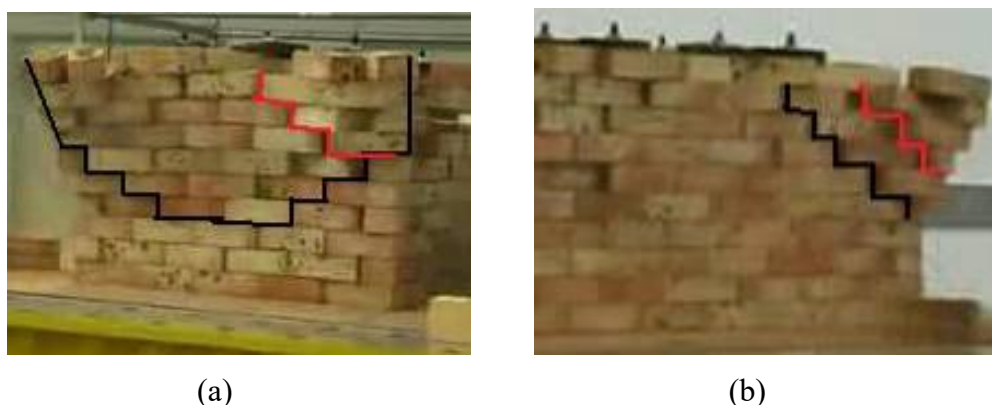
Figure 4.11 The response of Model I on x-axis 1.8Hz 12mm excitation ((a) the façade; (b) the side wall)
