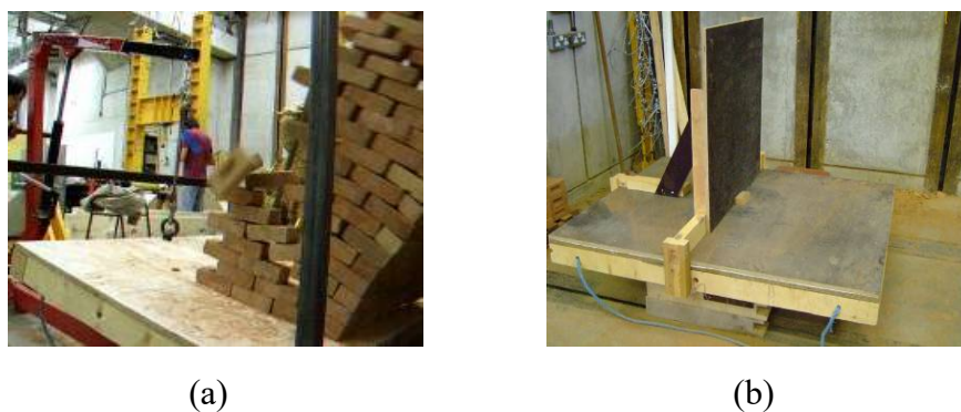
Figure 3.8 Experimental tests set up ((a) the tilting table; (b) the vertical board on the table)
