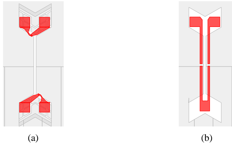
Figure 8.2 Redesigned ELOG templates, contact pads and sensing elements. Where (a) is a dual cantilever device with ‘grid-structured’ contact pad areas and (b) is a dual beam device with reduced size contact pad regions.
