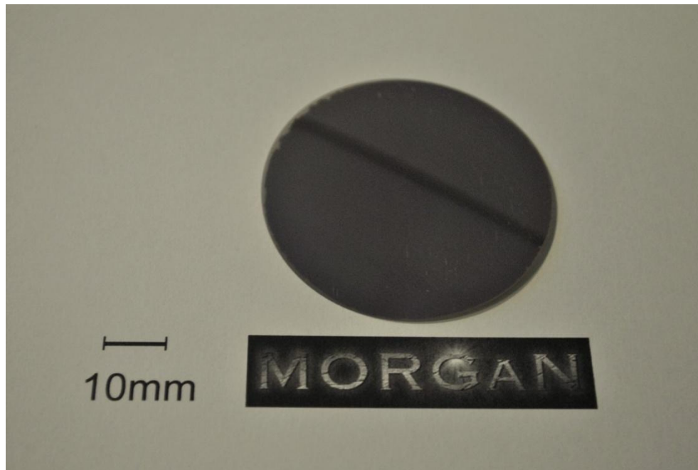
Figure 4.17 Image of a 2 inch (111) Si/PD wafer with a 2 \mu\text{m} Si device layer produced using hot KOH etching.
