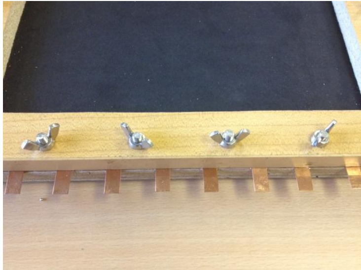
Figure 7.4: Demonstration of 8 electrodes on each side
