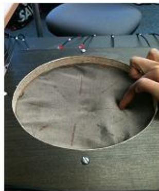
Figure 5.4: Pressure applied at the centre of the sensor
