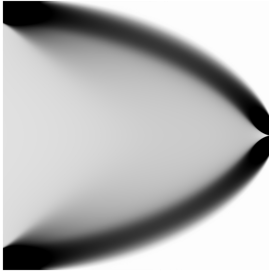
Figure 5-2: Solution of convex problem on a short cantilevered beam domain. The density of material is plotted with black colour denoting the presence of material with density x_i = 1 and white colours the representing the absence of material, i.e. density x_i = 0 . The colour scale is linear with the density of the material. This was solved using MMA on a mesh of 1600 \times 1600 elements.
