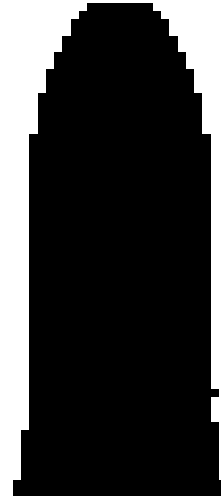
Figure 6-18: Solution computed on a mesh of 60 \times 60 elements. The buckling constraint is set to c_s = 0.5 and the compliance constraint c_{\max} = 5.5 . In this case, compared with Figure 6-17, the higher compliance constraint has led to a solution where this constraint is inactive and the buckling constraint is now active.
