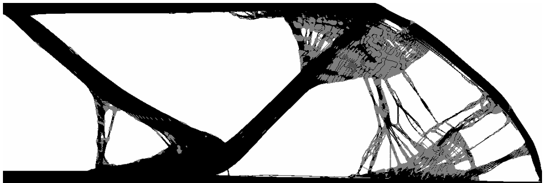
Figure 5-10: NAND SIMP solution to MBB beam on computational domain without filtering
