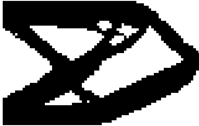
Figure 6-10: Solution found on mesh of 80 \times 50 elements. The buckling constraint is set to c_s = 0.9 and the compliance constraint c_{\max} = 60 . A volume of 0.5535 is attained. Here the buckling constraint c_2 is active and the compliance constraint c_1 is not.
