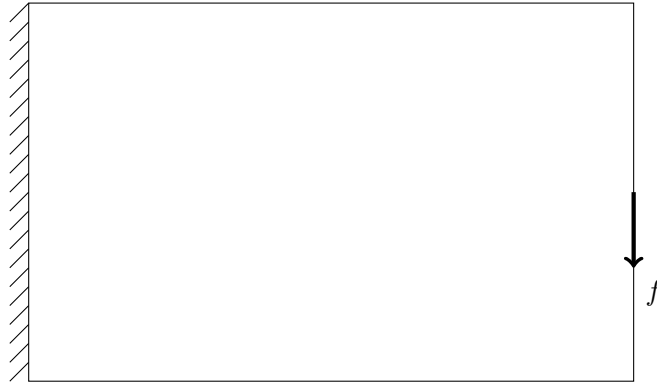
Figure 1-2: Design domain of the short cantilevered beam showing the applied load f and the fixed boundary conditions
