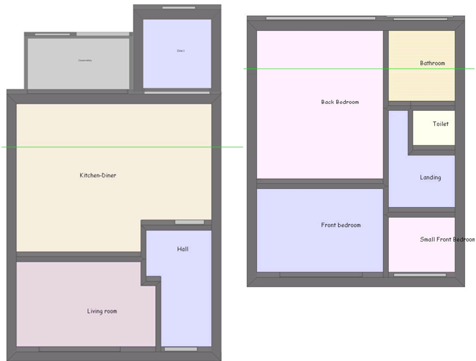
Figure 40 Plan layout of three-bedroom semi-detached house use to model hours of discomfort
