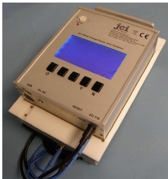
Figure 4.1 Image of the JCI 155v6 Charge Decay Time Analyser (reproduced with permission from JCI Chilworth Ltd.)
