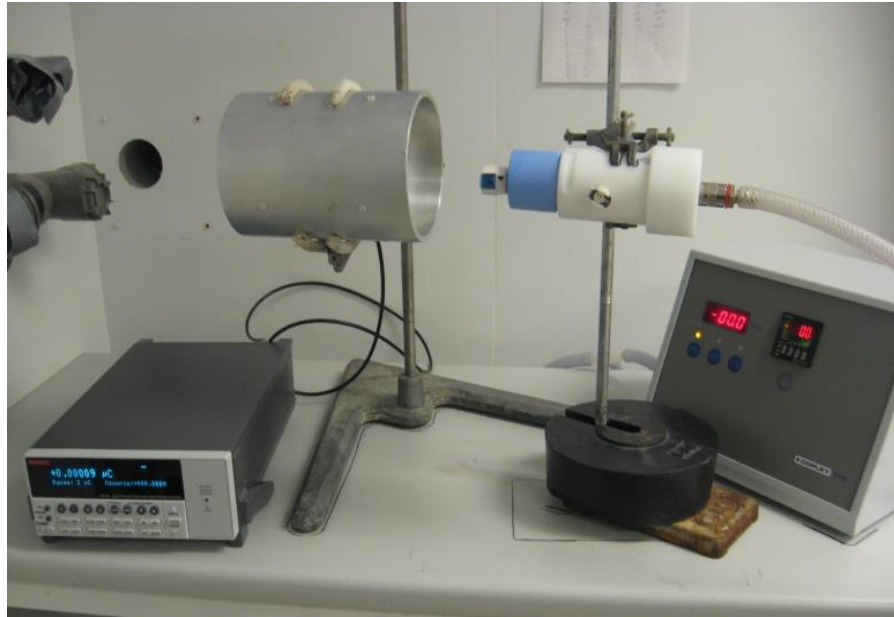
Figure 2.6 Experimental set up with electrometer, FTF, Aerolizer® device, DUSA and TPK
