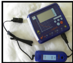
This is a Datalogger with a pulse rate sensor attached.
