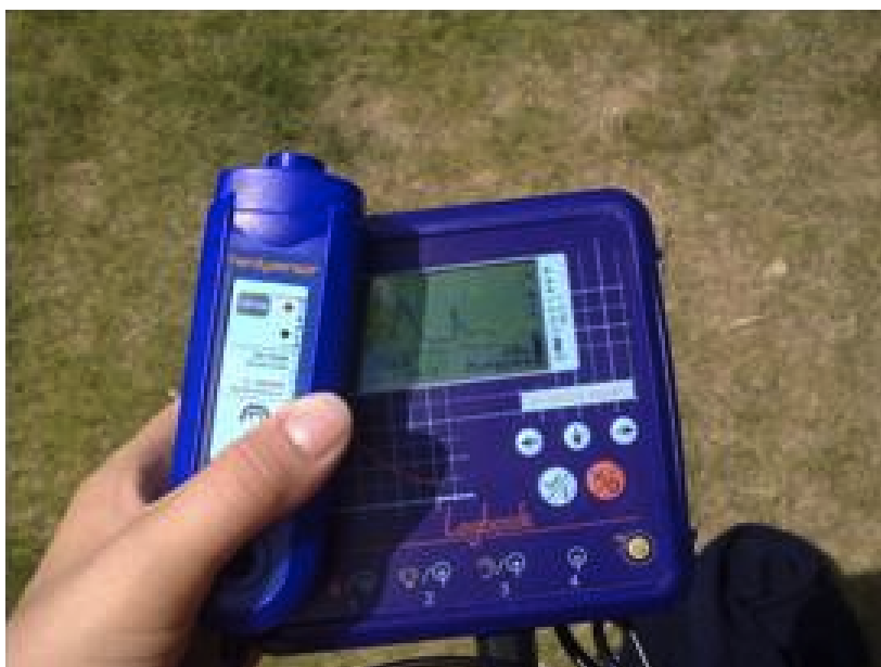
Figure 18.1: Logbook GL with additional Sound Sensor
