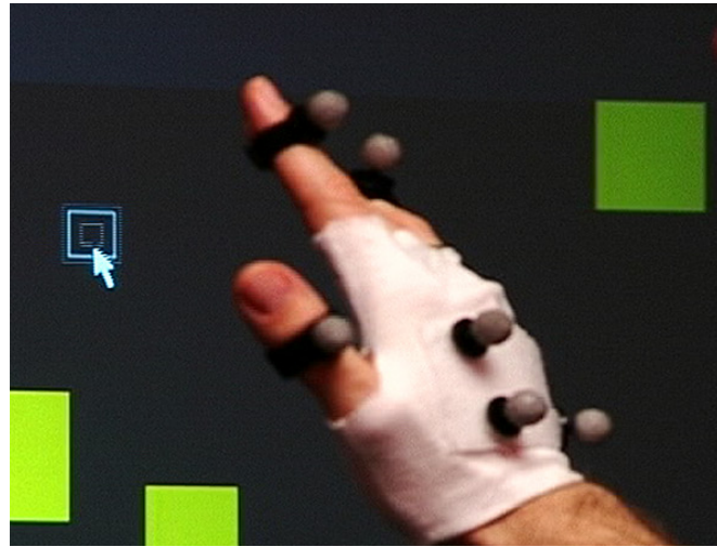
Figure 2-7: Vicon motion tracking system with passive markers attached to the hand [173].
