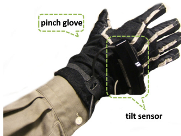
Figure 2-6: Glove device used for menu selection [127].
