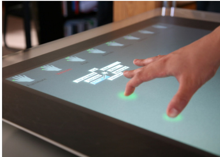
Figure 2-9: The multitouch marking menu [113].
