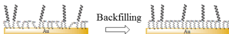
Figure 4.2 A backfilling step with MCH after an initial SAM formation provided a better reorganisation of the SAM structure.
