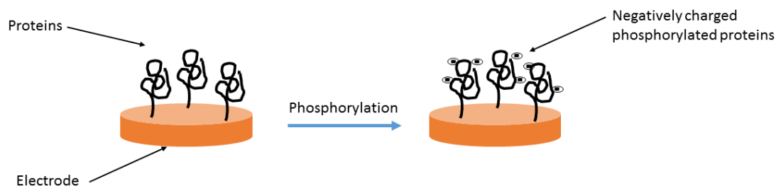
Figure 5.3 Protein monolayer transformation after phosphorylation reaction.
