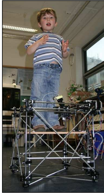
Figure 59: The strength of the design was tested by placing a small child (Johnny Adkins, 15.0 kg) on the Z-bed. Ian Adkins (father) used dedicated stepper driver chips with MOSFET technology to move Johnny up and down at a speed of 30 mm/s.
