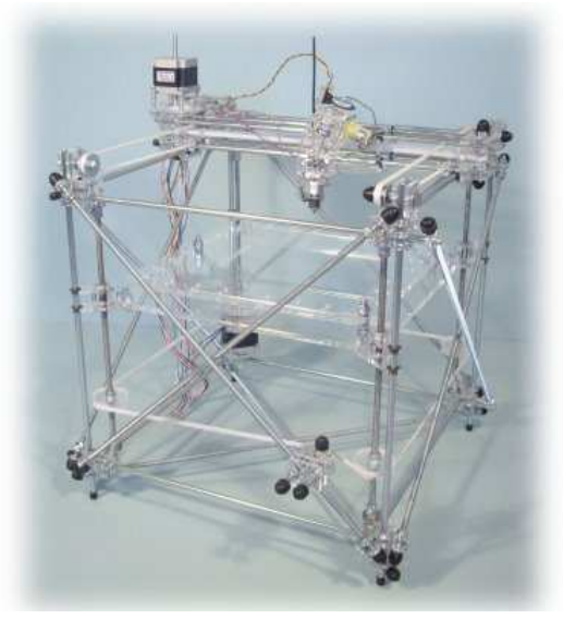
Figure 81: Evolution of Darwin's 'printed parts' design to enable them to be laser cut for a cheaper assembly.
