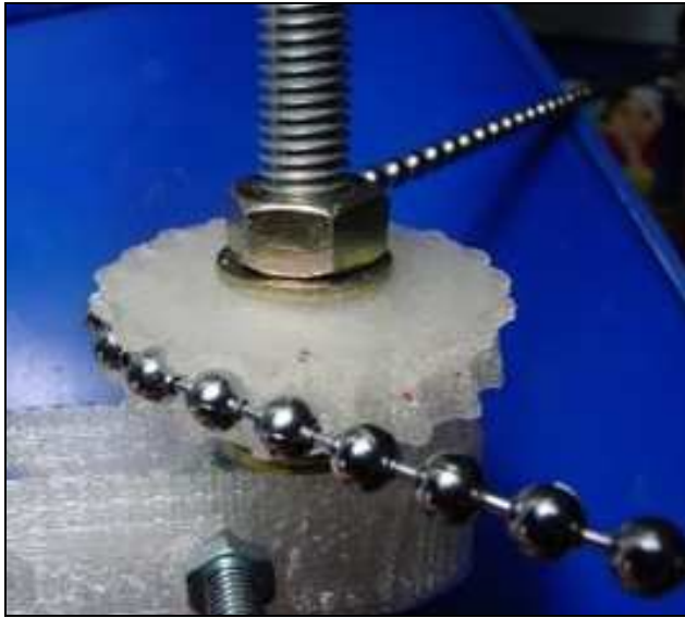
Figure 80: Evolution of Z axis transmission - the toothed belt has been replaced by a cheaper bath-plug ball chain.
