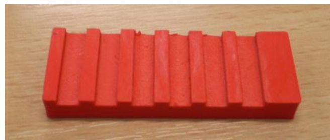
Figure 5.24 – Six slots of the total 36 slots in the dry slot milling experiments
