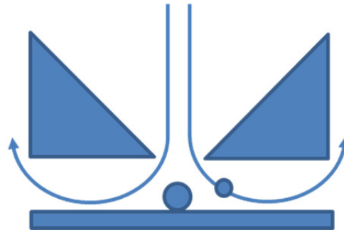
FIGURE 2.14 THE PRINCIPLE OF PARTICLE IMPACTION WITH LARGE PARTICLES UNABLE TO NEGOTIATE THE SUDDEN CHANGE IN THE DIRECTION OF AIRFLOW WHILST SMALL PARTICLES ARE CARRIED IN THE AIRFLOW
